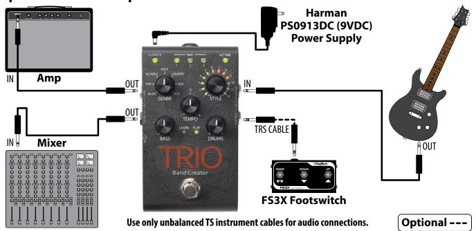
**NOTE:** When connected to both the MIXER and AMP OUT jacks, the guitar signal will be fed to the AMP output and the bass and drum parts will be fed to the MIXER output. See 'Output Jack Operation' on page 9 for more information.
