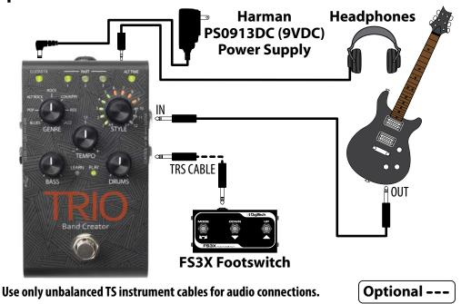
**NOTE:** When the HEADPHONE OUT jack is used, AMP and MIXER outputs will be muted. The signal present in the headphones will be stereo and speaker cabinet emulation will be applied to the guitar signal. See *'Output Jack Operation' on page 9* for more information.
